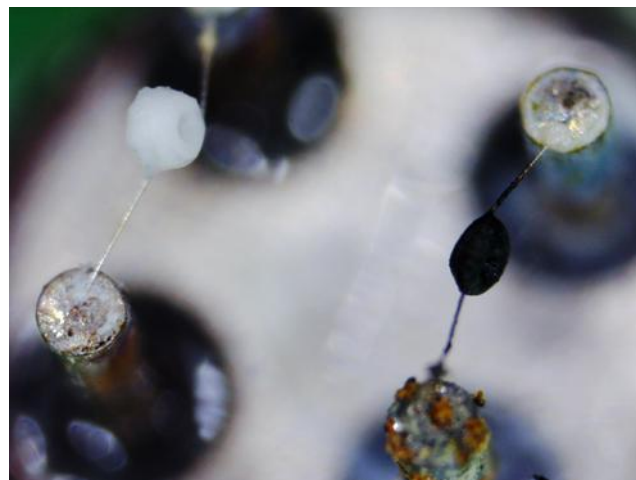
Fig. 1. Pellistor consists of working (black) and comparative (white) sensors.
